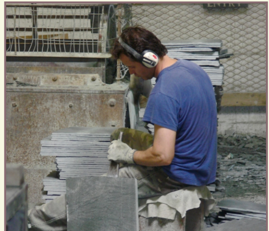
Slate being split along cleavage
